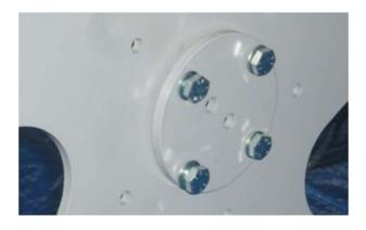
INSERT PLATE INTO BLADE SUPPORT USING SCREWS M10x45 TE NUT. 10,5x20 h2
