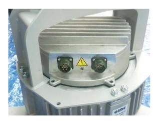
Lean Pc Board to connect power line and probe – ATTENTION to colours: U-BLACK/V-GREY/W-BROWNAssembly PC board to motor and clamp it.
