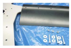
901484 SCREW M8x60 TCEI 901485 NUT 8,4x24 h2 901474 SELFBLOCKING BOLT M8
