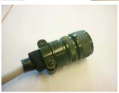
USE ARAOUND CABLE ONE SHEATH TO INCREASE THICKNESS AND HAVE OPTIMUM CLOSING
