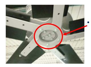
Fix without tightening the 5 central screws of the reinforced spider to the main one, with bolts and nuts
