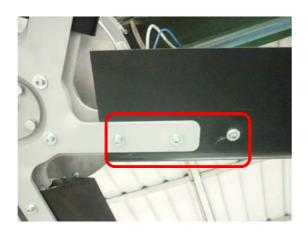
901484 SCREW M8x60 TCEI 901485 NUT 8,4x24 h2 901474 SELFBLOCKING BOLT M8
