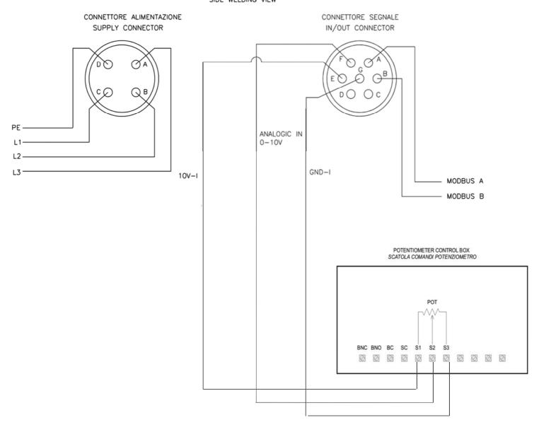
NB: It is necessary pull the A and B wires down to the control box for the Modbus connection, used for maintenance and diagnostic actions.
