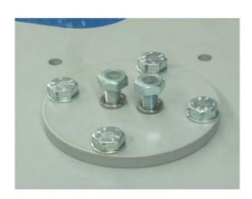
PLACE BLADE SUPPORT WITH DISC OVER THE SHAFT AND CLAMP SCREWS M10x35 TE WITH NUTS GROWER D.10
